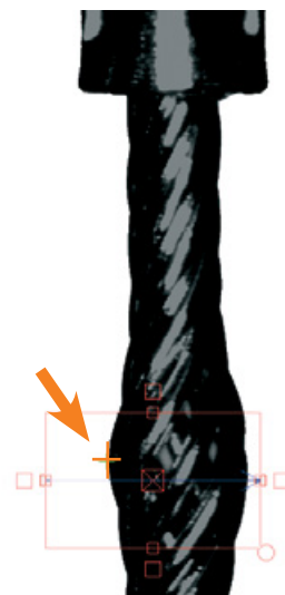
▲ EXAMPLE OF CONTACT INSPECTION
