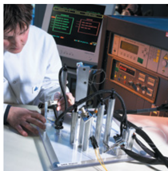
▲ AUTOMATIC CONTINUITY & INSULATION RESISTANCE TEST
