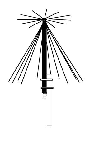
ColourStarFrequency Range225PolarisationVertGain+2dVSWR<2:'</td>Impedance (output)500Power Capability100ConnectionN tyOverall Dimensions410Mounting Pole Length340notWind Survival160Weight910
