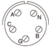
28-12, 28-13 Three phase AC, 4 wire, grounding
