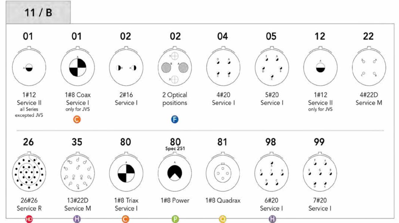
As stated in MIL-DTL-38999 standard, insert arrangements using multi-axial contacts (coax, twinax, quadrax, ...) should not be used in firewall applications.
