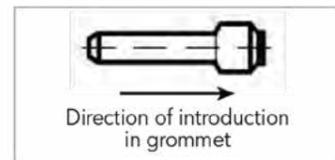
These filler plugs are installed at the rear of unwired contact to maintain connector sealing.
