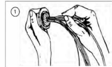
2 - Slide the tool down towards the contact. Insert the tool in the insulator until it abuts the contact shoulder.
