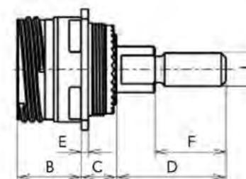
With 8D7 (jam nut receptacle)
