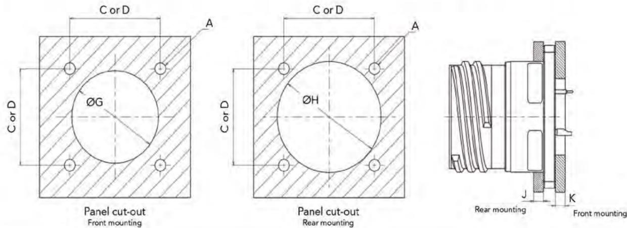
Note: All dimensions are in millimeters (mm)
