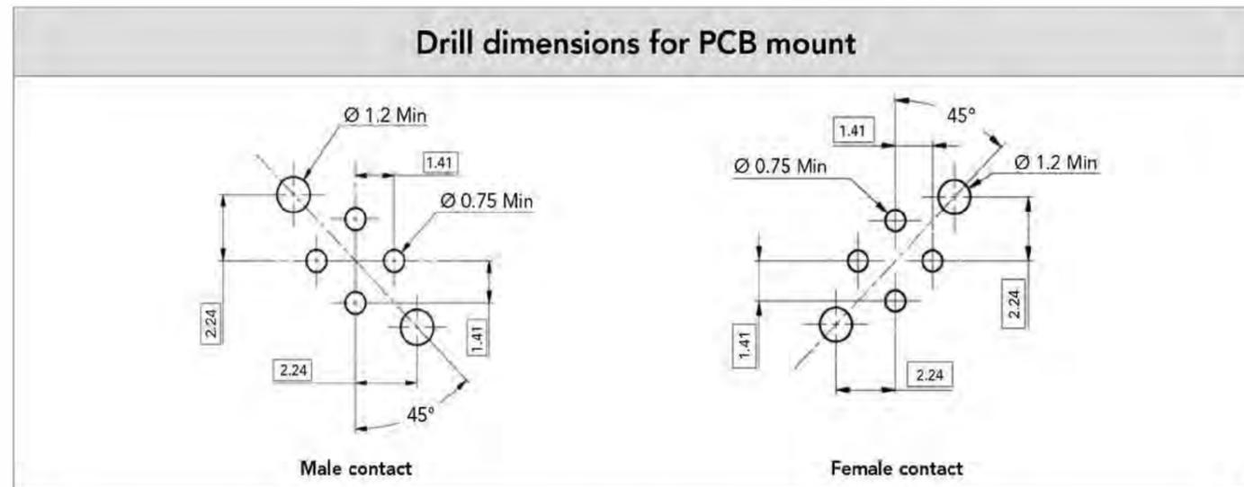
Note: All dimensions are in millimeters (mm)
