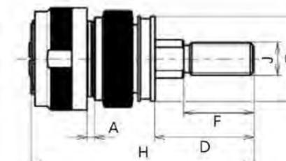
With 8D7 (jam nut receptacle)
