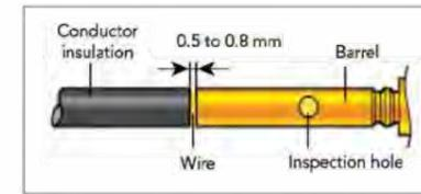
When inserting the stripped wire into the contact barrel check that no strands are left outside and that the wire is visible through the wire inspection hole in the barrel.
