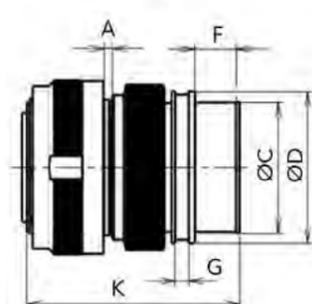
With 8D7 (jam nut receptacle)
