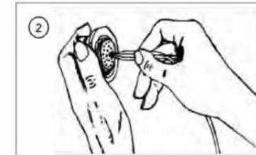
3 - Withdraw the tool from rear. Check that contact is firmly locked by pulling wire gently. When connector is fully loaded, check the position of contact tips. They should all be in the same plane. Nota: For larger sizes of cable which are stiff enough manual insertion without tool is preferable.
