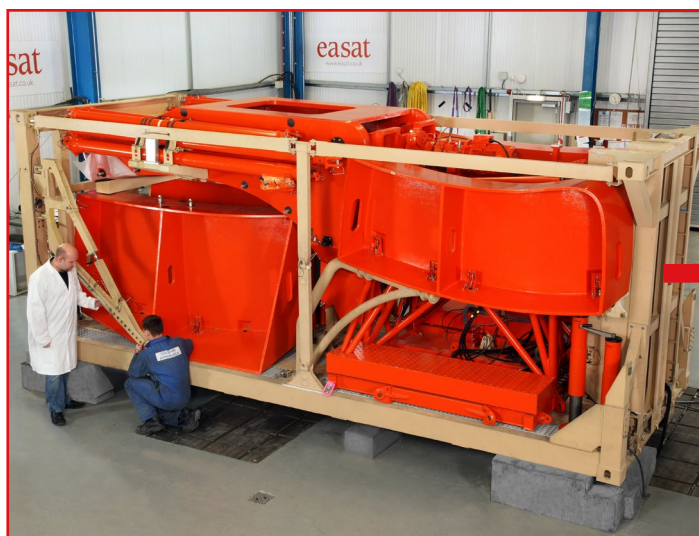
Easat Transportable ATC Radar shown in stowed / palletised configuration and in fully deployed configuration
