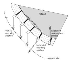
Designed for use on offshore oil and gas platforms and buildings
