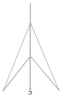
HF Band 2-30 MHz Length 9.5m (32ft) Pattern Omnidirectional
