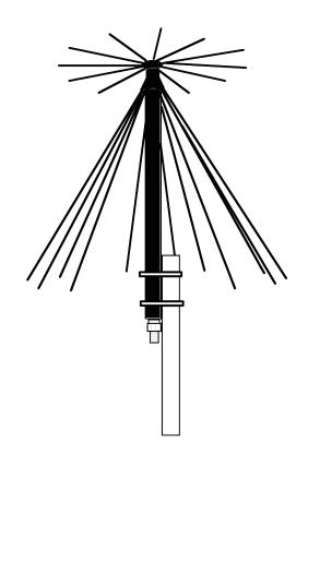
200MHz to 1500 MHz Vertical linear up to +2.5dBi over frequency range <3.5:1 over frequency range – typically better than 2:1  $50\Omega$  (nominal) Receive only N type coaxial connector (female) in base 800 (31.5 in) H x 900mm (35.5 in) Dia. 740mm (29.1 in), longer to order; mounting clamps not included 160 km/h (100mph) 2.2g (4.8 lbs); packed: 3.0kg (6.6 lbs)
